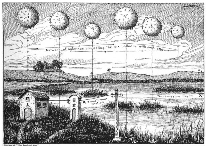
PLAUSON'S PROPOSED BALLOON PLANT FOR COLLECTING AND UTILIZING ATMOSPHERIC ELECTRICITY
